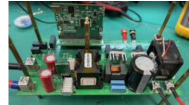
Benchmark For Server 1KW Solution
